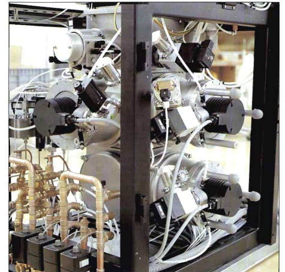
Fig. 10 The high-vacuum pumping station with its three TURBOVAC 1000 turbomolecular pumps
